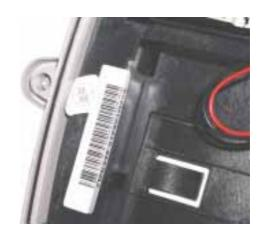
Verfication sealing in bottom of transmitter
